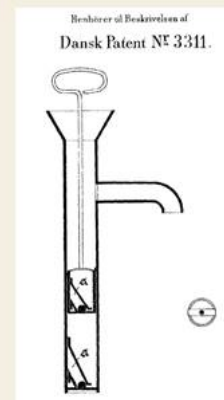
Anti-abrasion ball valve patented in 1900
